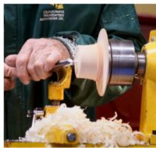
The depth inside of the crown was checked to ensure there was enough wood left at the top for finishing of the crown. The hat was then reversed and
