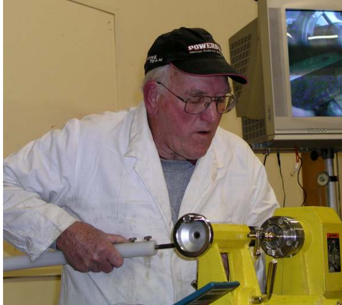
Rex Marshall's pewter-inlaid box Les Brindley turns brass on a wood lathe in April
