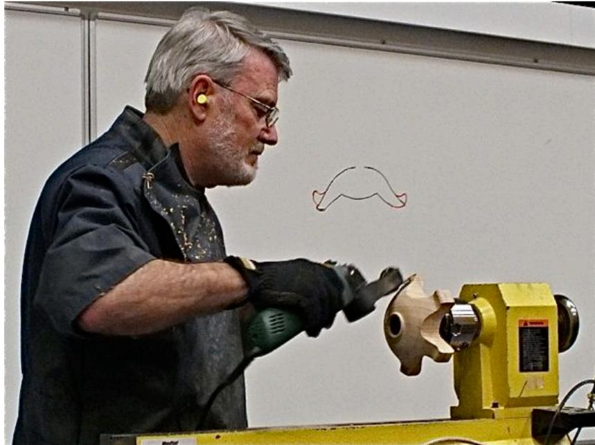
arboritech to remove the timber to get the right feet up and down. To illustrate how important it is to pre-mark the job, he nearly lopped the wrong foot. The arboritech with another blade left a smoother finish and refined the shape.
