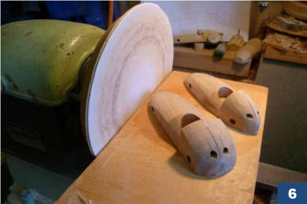
Figure [6]: Shape the chassis to final form. A sanding disc makes short work of this job. Aim for nice, flowing curves in plan and profile to give them that classic racer look, but take care as it's easy to remove too much material.
