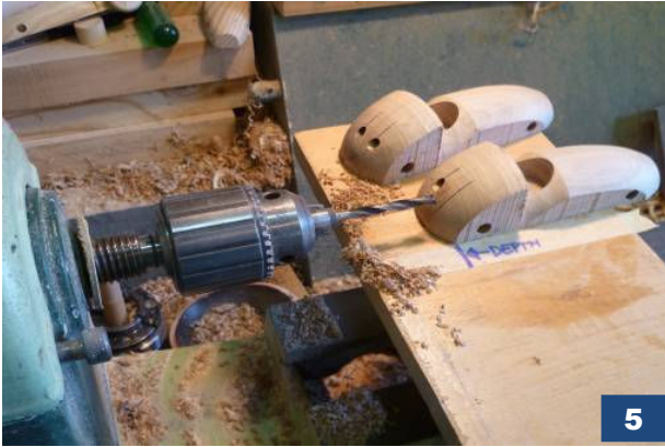
Figure [5]: Drill 6mm holes for the exhaust pipes at this stage, before final shaping of the rear chassis. A brad-point drill makes starting the hole on the sloping face a little easier.
