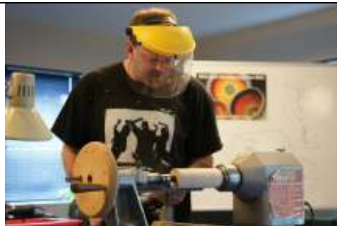
Neck hole drilled with forstner bit then rim shaped with bowl gouge
