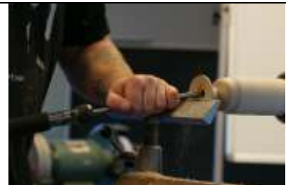
Neck hole drilled with forstner bit then rim shaped with bowl gouge
