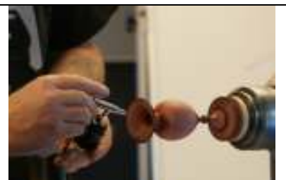
Fine shading is applied by airbrush (Sprit based dye) using 30psi
