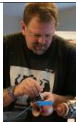
Air pressure turned down to 20psi so dye is not blown under template
