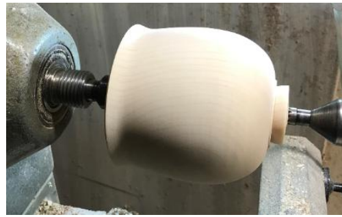
Rough out form and cut tenon for chuck mounting
