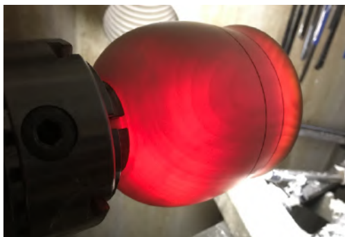
Using a light to gauge uniform thickness
