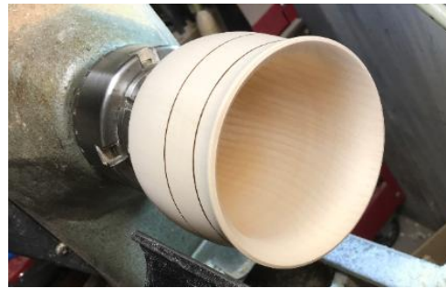
Rough out form and cut tenon for chuck mounting
