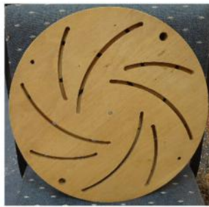
Longworth Chuck under construction
